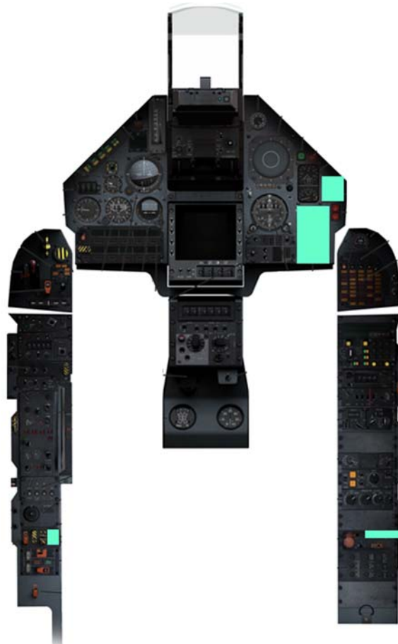
Figure 2 Fuel panels locations
