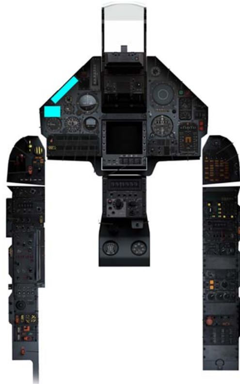
Figure 11 Autopilot panel location
