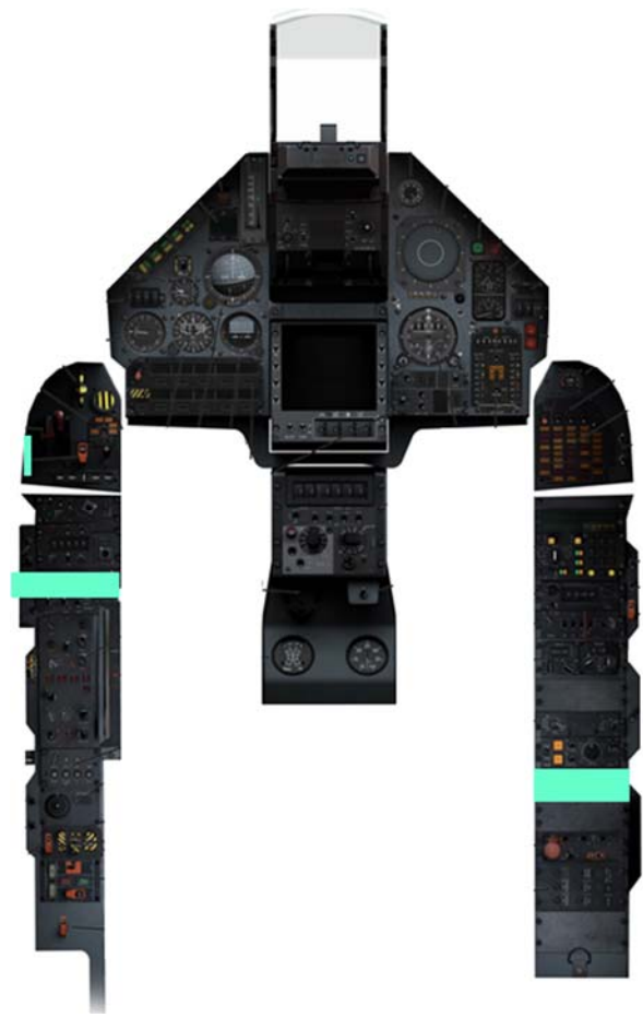
Figure 5 Internal and External lights panels
